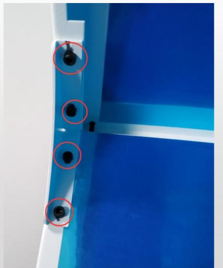
10. Find the front plate (<u>label: front-G</u>), install the hinge (fixed with 4pcs M5X10 screws), install the door handle (fix with 2pcs M4X6 screws), Install magnets, arrange two 20X10X5 magnets side by side inside the door.
