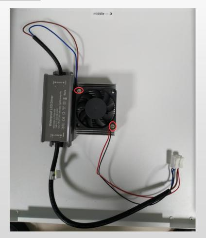
6.Connect the cable: one end of the cable has been connected to the terminal, need to connect the two wires reserved on the top plate. (There are two types of terminal blocks)
