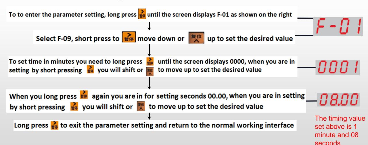
Note: seconds setting, the two digits on the left represent the tens digit and the ones digit respectively, and After the two digits on the right represent the decimal point, the set value will not be displayed on the panel.
