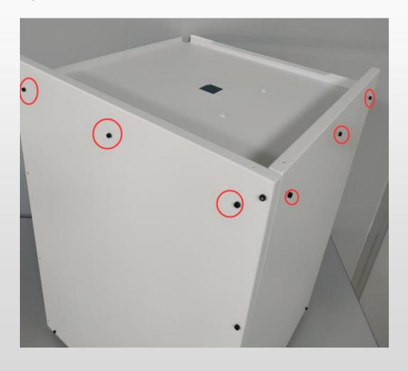
4. Find the right plate (<u>label: right-E</u>), use 7pcs M3X20 screws to fix it to the bottom plate and the back plate, and use 3pcs M3X6 screws to fix it to the middle plate.
